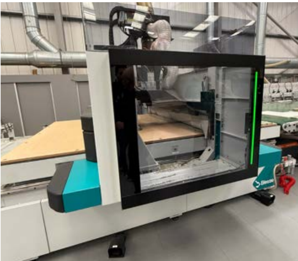
Accurate cutting of plywood, MDF and timber components directly from digital files.
